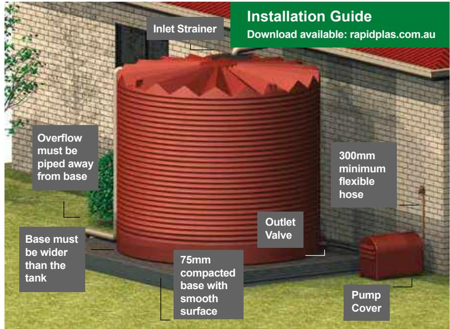
NB: 1mm of rain falling on 1m<sup>2</sup> of roof area gives you 1 litre in your tank.
